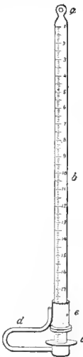
The Niche Evaporimeter. a , eye by which tube is suspended; b , tube containing water; c , disk of paper kept in place by a metallic spring; d , attached to a slotted collar; e , that moves along the tube. Each scale number corresponds to a cubic centimeter of water or the evaporation of a layer .0264 inch deep, from a free water surface in the instrument-shelter.
