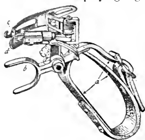
Barber Knotter. a, strap for fastening on the hand; b, thumb-piece; c, knottor and cutter; d, thread-guide.
