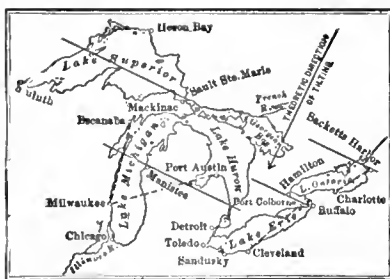
Map of the Great Lakes, showing pairs of gaging-stations and isobases of outlets. The isobases are marked by full lines; broken lines show the pairs of stations.
