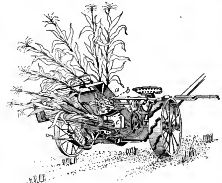
Corn-binder. a, guides for bringing the stalks to the knife (not shown); b, binding-mechanism; c, bundle of stalks ready to be discharged.
