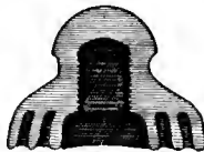
Cross-section of a Triple-petticoat Insulator.
