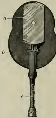
Loring's Ophthalmoscope. a , mirror; b , body; c , shank, into which the handle (not shown) is screwed.
