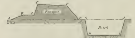
A, foot of banquette slope; B, crest of banquette; C, interior crest; D, foot of interior slope; E, exterior crest; F, foot of exterior slope; G, crest of scarp; H, foot of scarp; I, foot of counterscarp; J, crest of counterscarp. AB, banquette slope; BC, banquette tread; CD, interior slope; CE, superior slope; EF, exterior slope; FG, berm; GH, scarp; HI, bottom of ditch; IJ, counterscarp.
