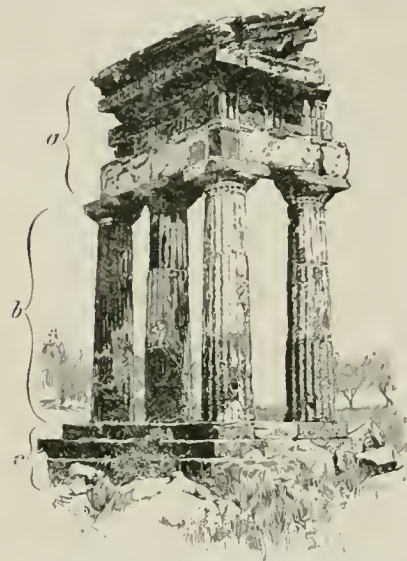
Doric Order.—Temple of Castor and Pollux (so called), Gigenti, Sicily. a, entablature, consisting of cornice, frieze, and architrave; b, column, consisting of capital and shaft; c, stylobate, which in the Doric order performs the function of a base.
