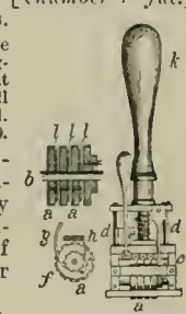
Numbering-stamp. a, numbering-wheels each with ten Arabic figures, 1 to zero inclusive; b, arbor on which the wheels turn; c, frame which carries the arbor and wheels; d, guides rods on which the frame c slides; e, spring which is compressed by the frame in stamping; f, ratchet-wheel with ten teeth corresponding to the ten Arabic figures, 1, 2, 3, etc., to 9; g, spring-pawl, which, on the spring being compressed, engages the tooth of the ratchet-wheel next to that previously engaged; h, another spring-pawl, which prevents back motion; i, handle; j, intermediate carrying-mechanism.
