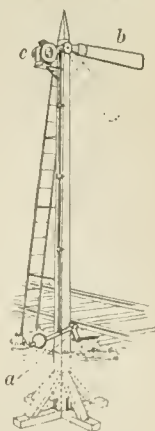
Railway Semaphore. a, lever, which operates both a, blade, and c, lantern.
