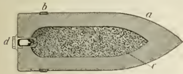
Shell for use in Army and Navy Breech-loading Rifled Ordnance. a, body of shell, of cast-iron for ordinary use, or of steel for penetrating armor; b, rotating ring of copper, which engages the rifling-grooves and imparts axial rotation to the shell; c, powder-charge; d, Hotchkiss percussion fuse.
