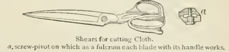
Shears for cutting Cloth. a, screw-pivot on which as a fulcrum each blade with its handle works.
