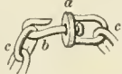
Swivel. a, swivel; b, hook, turning freely in a; c, c, chain.
