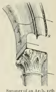
Summer of an Arch, 12th century. 2 summer. (From Viollet-le-Duc's "Dict. de l'Architecture.")
