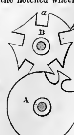
The Geneva Stop Movement, used in Swiss watches to limit the number of revolutions in winding up, the convexly curved part, a , b , of the wheel B serving as the stop.
