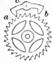
Pallet, 7. a and b are the pallets of an anchor-escapement which oscillates on the pivot c.
