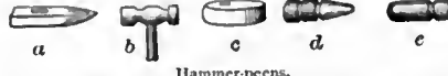
Hammer-peens. a, narrow peen for riveting; b, broad peen for machinists; c, cross-peen for coopers; d, cone peen for chasing; e, ball peen, upsetting hammer for engravers.
