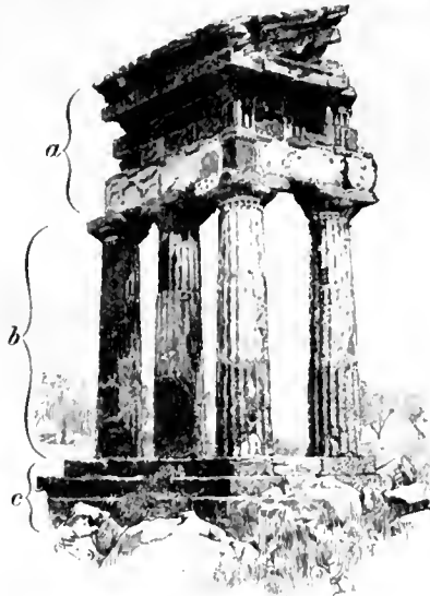
Doric Order.—Temple of Castor and Pollux (so called), Gigenti, Sicily. a, entablature, consisting of cornice, frieze, and architrave; b, column, consisting of capital and shaft; c, epistyle, which in the Doric order performs the function of a base.
