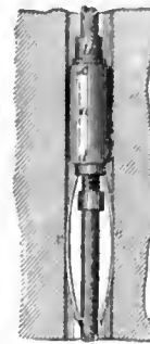
Oil-well Packing. a, an elastic substance surrounding the main tubing; b, the ordinary coupling resting on the washer c, their surfaces ground together and made water-tight; d, a loose nut running upon a screw-thread cut on the main tubing; e, elliptic springs, dovetailed or otherwise fastened to the sides of the loose nut d, and partially clamping the tubing at f.
