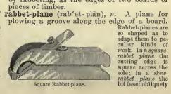
across the sole; in a side-rabbet plane like cutter is on the side, not on the sole. rabbet-saw (rab'et-sâ), n. A saw used for mak-
