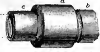
a , reducer, connecting the pipe of larger diameter b with the pipe of smaller diameter c .
