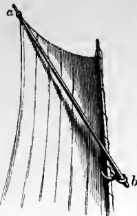
Snotter (b). a, sprit with the lower end in the snotter (a).
