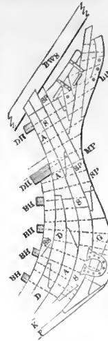
Stem and allied parts. S, stem; K, keel; A, apron; D, deadwood; SS, stenson; DH, deck-hooks; BH, breast-hooks; ST, stem-piece, or independent piece; MP, main piece, or lace-piece; BP, bobstay-piece; BWS, bowsprit; G, gripe; F, false keel. (The dotted lines show bolts.)
