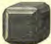
Bevelment of the edges of a cube by planes of a tetrahedron.
