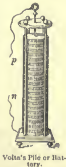
Volta's Pile or Battery. p, positive wire; n, negative wire.
