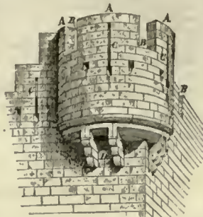
Bartizan.—Carcassonne, France. A, merlon; B, embrasure; C, loophole; D, machicolation. (From Viollet-le-Duc's "Dict. de l'Architecture.")
