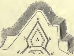
A. Bastion. a, a, curtain-angles; b, b, shoulder-angles; c, c, salient angle; a, b, a, b, flanks; b, c, b, c, faces; a, a, gorge; a, d, a, d, parts of curtains.
