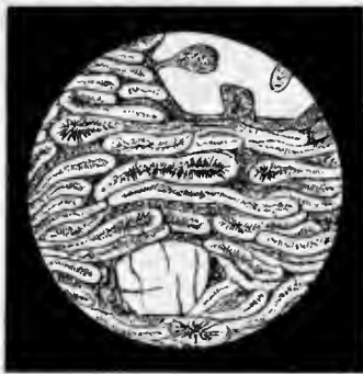
Axiolite.—Specimen of rhyolite from Virginia Range, Nevada, magnified 200 diameters. (From Zirkel's "Microscopical Petrography.")
