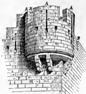
Bartizan.—Carcassonne, France. A, merlon; B, embrasure; C, loophole; D, machicolation. (From Viollet-le-Duc's "Dict. de l'Architecture.")
