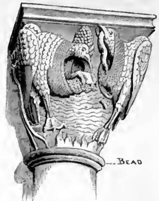
Bead as used beneath a capital.—Abbey-church of Vézelay, Yonne, France; 12th century. (From Viollet-le-Duc's "Dictionnaire de l'Architecture.")
