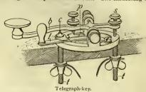
ton is held by the thumb and first two fingers, and stops are arranged to control the play or movement of the lever. The two ends of a bresk in the line-wire are connected to the terminals t, t, and the break is bridged over by the lever b each time it is depressed during the transmission of the message. When the key is not being used the lever is held against its bsck-stop s by the spring p, and the break is bridged over by putting the lever t in the position shown.
