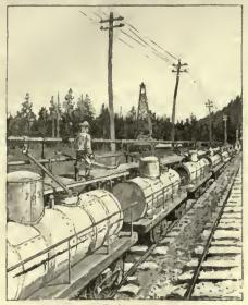
adapted for the transportation of petroleum in bulk. Sometimes eafled oil-car.
