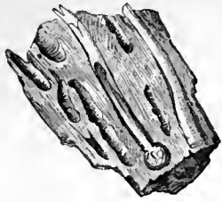
Piece of Wood Perforated by Teredos.
