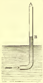
Pitot's Tube. A, tube; B, line to which water is raised by the force of the current.
