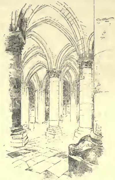
Vaulting.—Perspective of Vaulting as applied in a double curved apsidal aisle, Church of Notre Dame, Paris.
