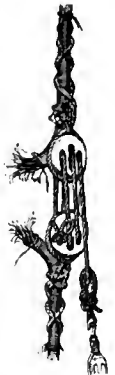
Fighting-stopper in place to secure a shroud which has been shot away.
