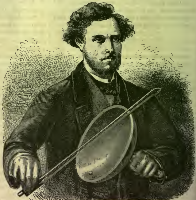
VIBRATIONS OF A METAL BELL.
