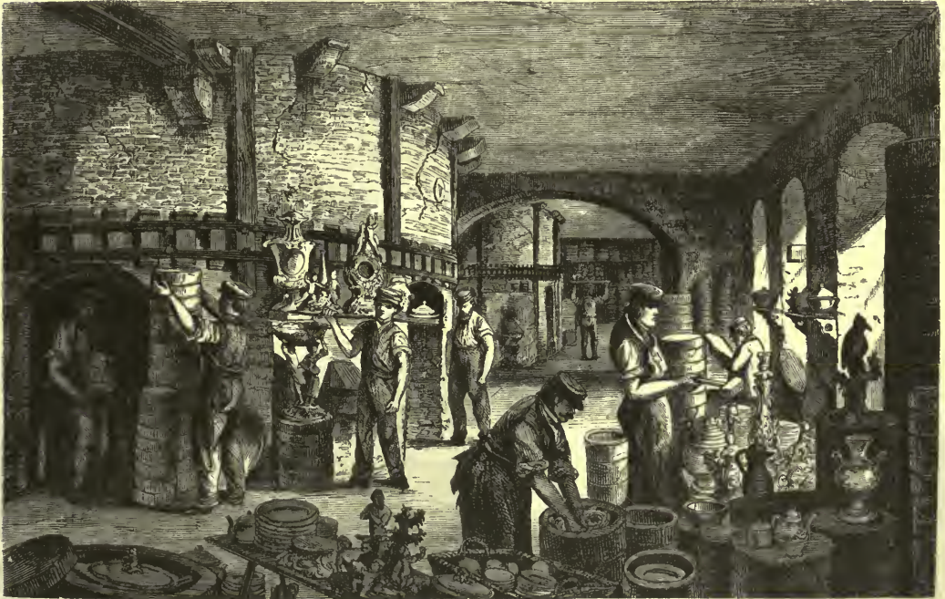
REMOVING THE BATCH FROM THE OVENS AND THE SEGGARS.
