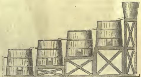
"FLOATING" GRAPHITE THROUGH THE TUBS.
