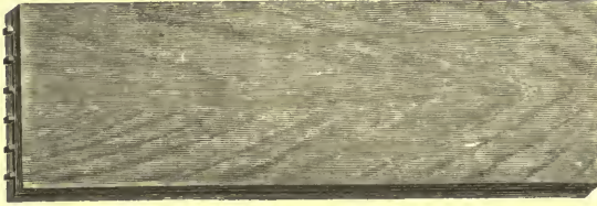
SLIPS SHOWING PENCILS IN SEVERAL STAGES OF PROGRESS: THE SINGLE SLIP, PARTLY FILLED; THE FILLED AND GLUED SLIP, ONE END SMOOTHED.
