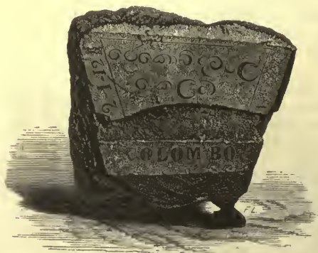
LARGEST PIECE OF NATIVE GRAPHITE EVER SHIPPED FROM CEYLON, WITH CINGALESE INSCRIPTION. WEIGHT, 237 LBS.
