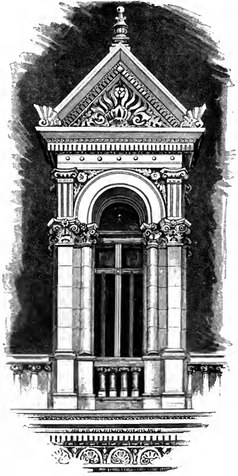
DORMER, STREET SIDE.
