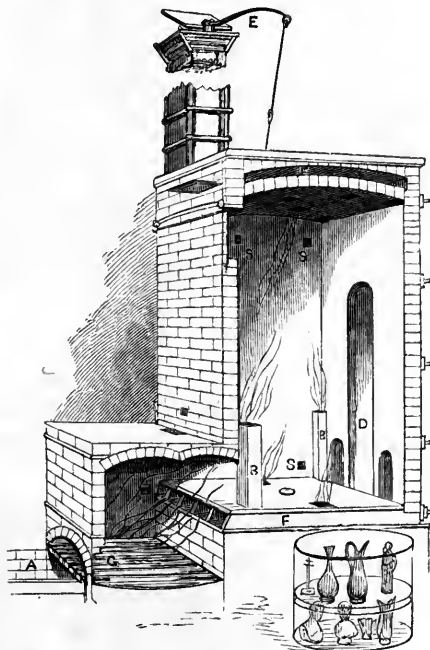
Fig. 29.—Broome's Improved Porcelain or Partian Kiln. A, ash-pit; G, grate; F F, flues; B B, bags for the flames; D, door for filling the kiln; E, damper, or draught regulator; S S S, spy-holes for watching, or trials while burning.
