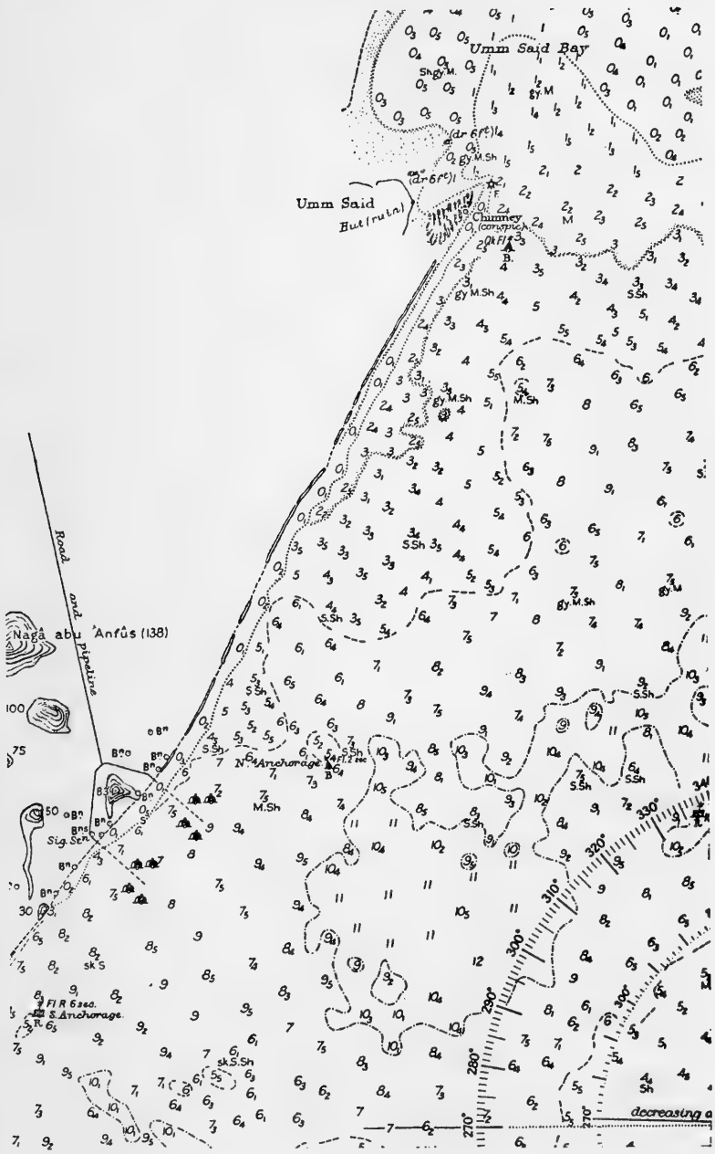
Portion of Admiralty Chart 3787, published 9th April, 1948, from the survey by H.M.S. Challenger. The pipeline and mooring buoys at the oil export terminal of Umm Said are shown.
