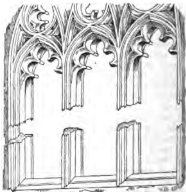
Mullion : Window from Carlisle Cathedral.
