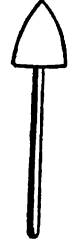
Fig. 1.—Push-pick: galleries are supposed to advance one foot and a half per hour; while with frames, the progress is barely more than half that amount.
