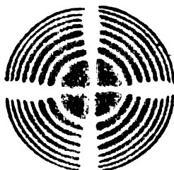
Fig. 3.—Uniaxial Crystal; White Cross.
