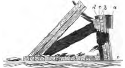
Fig. 3.—Section of do., showing the hole made by the 600-lb. shell, and displacement of the upper plate. a, armour plating, 4½ in. thick (displaced); b, teak backing, 18 in. thick; c, boiler-plate skin, ¾ in. thick; d, wrought-iron beams; e, platform.
