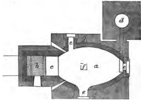
Fig. 2.—Plan of a Reverberatory Lead Furnace : a , hearth on which the ore is spread; b , fireplace or grate; c , the fire bridge; d , chimney; e , working doors; f , opening for supplying ore; g , tap-hole.
