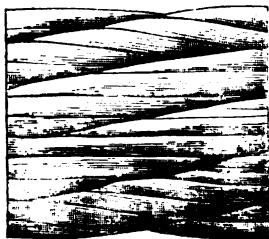
Section and External Appearance of Atlantic Cable of 1866.
