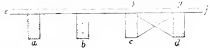
a, b, c, d , the joists; e, f , the flooring-boards; g and h , herring-bone strutting.
