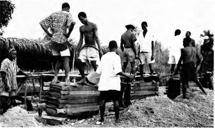
In labor intensive diamond mining operations, the gravel is excavated (top), put through foot shakers for sizing (middle), and washed (left) so that the diamonds can be picked out by hand. (Fig. 5)
