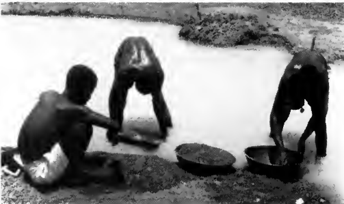
In labor intensive diamond mining operations, the gravel is excavated (top), put through foot shakers for sizing (middle), and washed (left) so that the diamonds can be picked out by hand. (Fig. 5)
