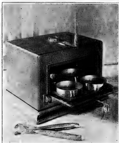
Fig. 18.—Steam ovens can be obtained of large or small size, holding 1 to 30 dishes, suitable for large warehouses or small factories.
