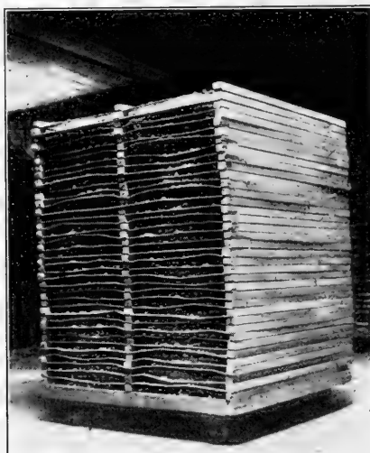
Fig. 21.—Drying trays on a wheeled truck permit the rapid drying of casein in large quantities, in a current of warm air.
