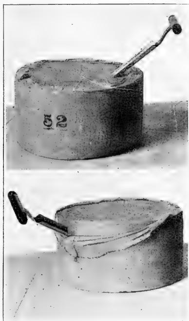
Fig. 44.—Cheese Sampling. Old cheese are sampled as shown in the upper figure. Cheese are sampled after dressing as shown below.
