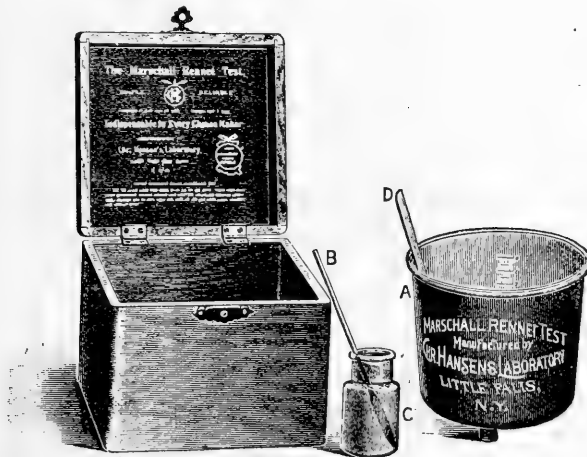
Fig. 12.—Marschall Rennet Test. The most convenient and widely used form of rennet test.
