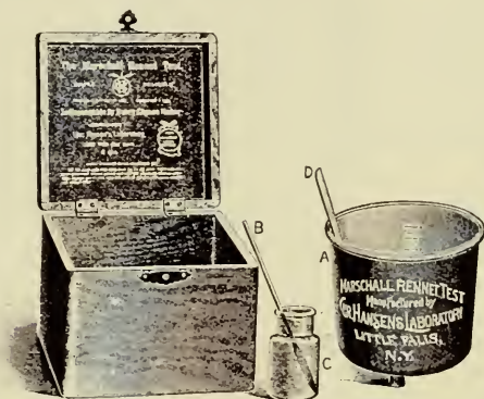
A—Graduated Cup. B—1 c. c. Pipette. C—Glass in which to dilute the rennet. D—Spatula for stirring the milk.
