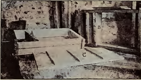
Block Swiss moulds. A, the adjustable end, moved by a screw. B, the partition which fits into the grooves, making the right sized molds after the blocks are cut. C, the cover or follower.
