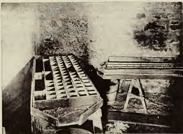
Limburger molds on pressing table, showing the long pieces and the short partitions between.
