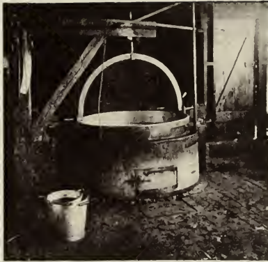
Swiss kettle in the Raub factory, near Monroe, Wis. The kettle hangs on a heavy wooden crane. The front of the fireplace over which the kettle hangs also hangs on a crane and can be swung out so that the kettle can be swung away from the fire. The opening below the grate will be seen in front of the kettle. The round cover is dropped over the top when the kettle swings forward.
