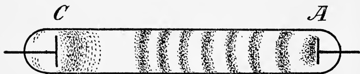
FIG. 47. ELECTRIC DISCHARGE UNDER REDUCED PRESSURE. C = Cathode. A = Anode.
