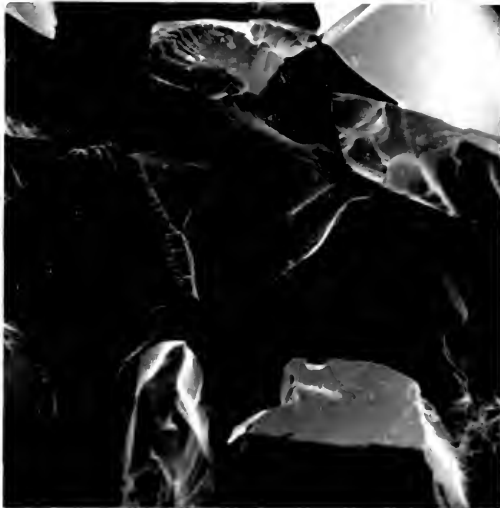
Figure 68. Scanning electron micrographs for -60+100 mesh NCS-1510 glass powders (a) corroded (1000X), and (b) corroded 3 days at 100°C (1000X).
