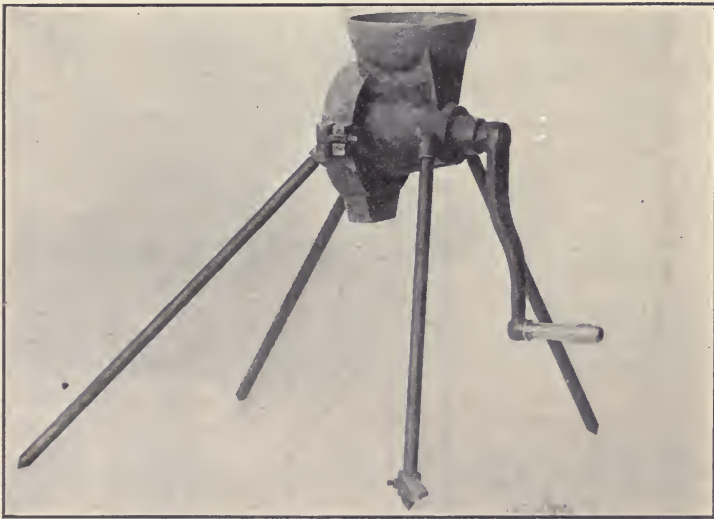
Figure 7—COAL GRINDER OF THE COFFEE-MILL TYPE Weight about 16 pounds. Readily knocked down for packing. Especially Designed for use in taking Face Samples.
