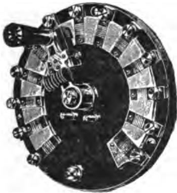
Storage Battery regulating Switch.
