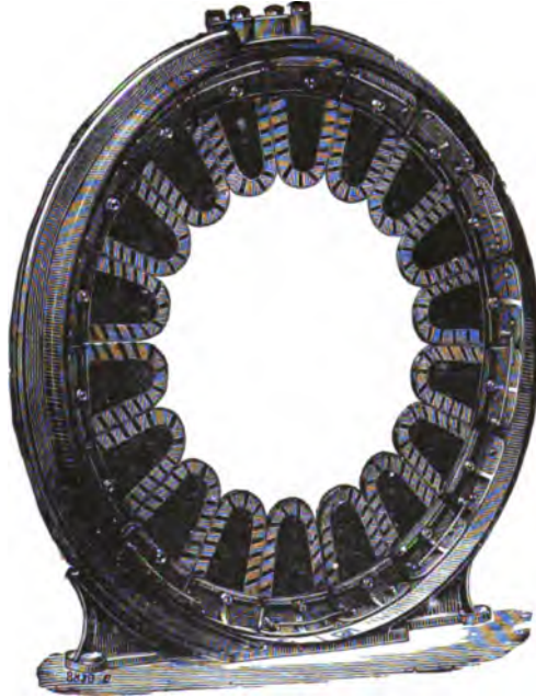
Armature of Mordey Alternator.
