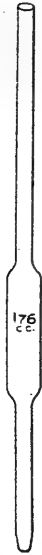
FIG. 3.—Pipette holding 17.6 cubic centimeters, used in measuring milk in the Babcock test.
