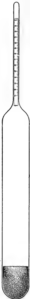
FIG. 31.—Special lactometer described in Bulletin 134, Bureau of Animal Industry, U. S. Department of Agriculture.
