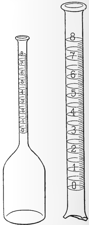
FIG. 2.—Type of Babcock milk-test bottle conforming to the requirements of the United States Bureau of Standards, and showing graduations.
