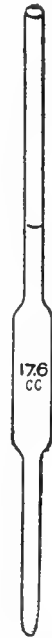
FIG. 3.—Pipette holding 17.6 cubic centimeters, used in measuring milk in the Babcock test.
