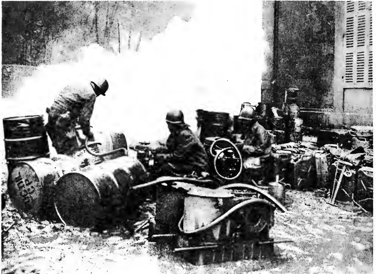
M2 SMOKE GENERATOR
