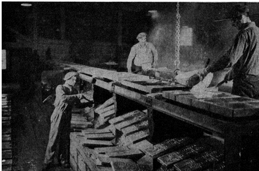
FIG. 27-4.—Liquid zinc is poured from a ladle into flat molds. Most of this metal will be used to protect iron.
