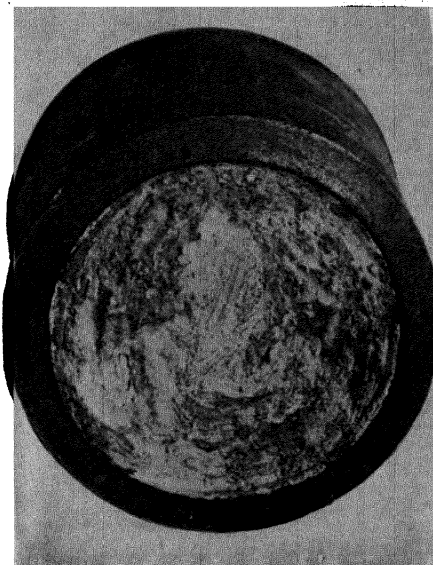
FIG. 35-3.—This steel boiler tube was completely filled with hard scale from hard water.
