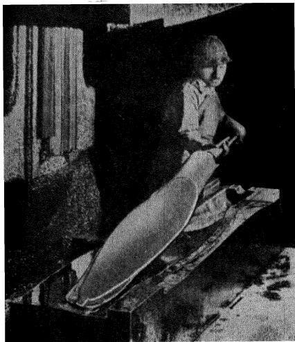
FIG. 26-6.—Forging an aluminum-alloy propeller blade is a convenient way of rough-shaping the metal.
