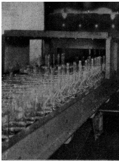
FIG. 16-2.—Borosilicate glass is made from sand, borax, and other materials. The first two important ingredients are found as natural minerals, silica and kernite. The glassware shown here is passing into an electric annealing oven.
