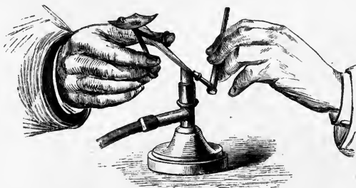
Fig. 112.—Fusion on platinum foil.
