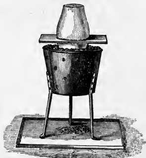
Fig. 210.—Extraction of arsenic.
