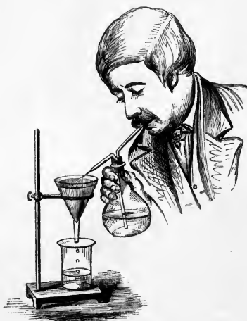
Fig. 115.—Washing a precipitate.
