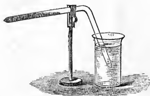
Fig. 129.—Liquefaction of ammonia.
