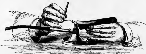
Fig. 107.—Reduction of metals on charcoal.
