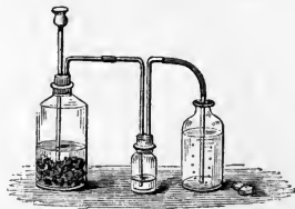
Fig. 186.—Preparation of hydrosulphuric acid.
