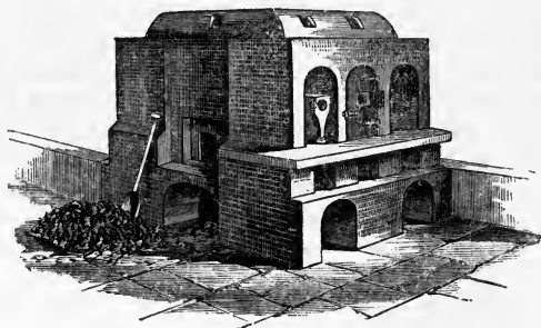
Fig. 228.—Silesian zinc furnace.
