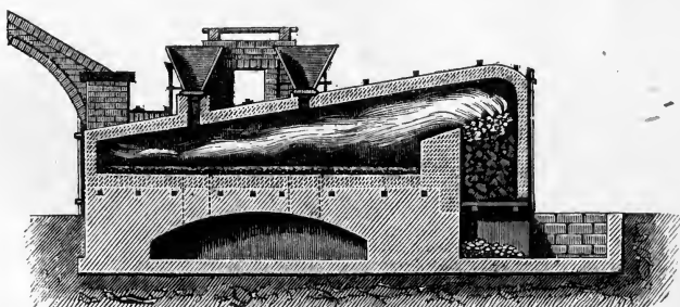
Fig. 76.—Reverberatory furnace for copper smelting.
