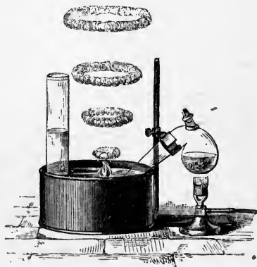
Fig. 209.—Preparation of phosphuretted hydrogen.
