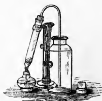
Fig. 146.—Preparation of nitric peroxide.
