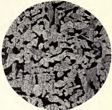
2. Steel about 0.30 per cent. carbon. 100 Diams.
