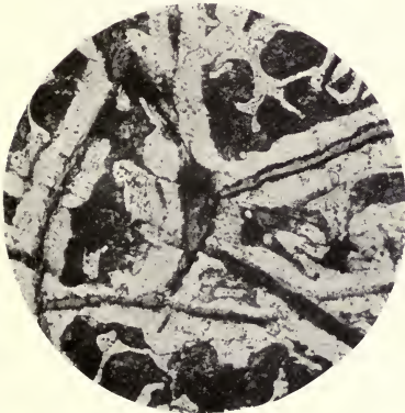
7. Gray cast iron, No. 2 foundry. 100 Diams.
