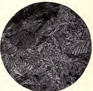
4. Steel eutectoid, 0.85 per cent. carbon. 400 Diams. (note homogeneity).
