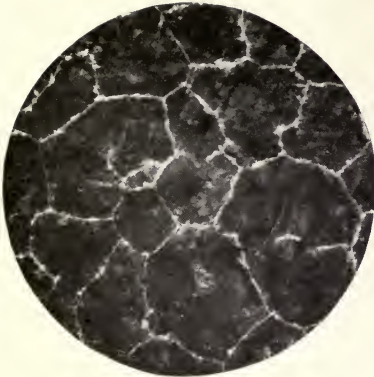
5. Steel hypereutectoid, 1.10 per cent. carbon. 100 Diams.
