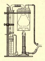
method. By this means the volatile portion seems to distil more readily, and after completing the determination the flask is more easily cleaned. The graduate is weighed, and when all water and benzine have distilled over, the graduate and contents are weighed and the increase in weight equals water and benzine. The weight of water in grams is equal to the c.c. present, and the difference equals benzine.
