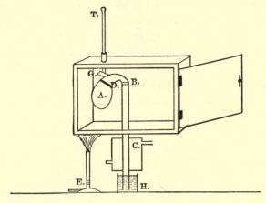
consists of a copper retort A, of about 200 c.c. capacity, detachable at D to admit of filling and subsequent cleaning. G is a small opening for admission of coal gas. (This may be dispensed with, but when used it should be freed from moisture by passing through CaCl<sub>2</sub>.) The copper tube leading from the retort is connected at B to the glass condenser C. A copper oven, open at the bottom excepting for a covering of copper gauze, is fitted over the apparatus as shown. It contains
