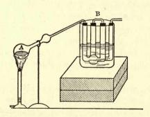
verized sample in the flask A, and pour over it concentrated HCl. At once connect A to B, in which is a solution of KI, the containing tubes being kept cool by filling the beaker about one half full of water. Now apply a burner to A and heat the solution until the sample is completely dissolved and all the evolved chlorine has been expelled and
