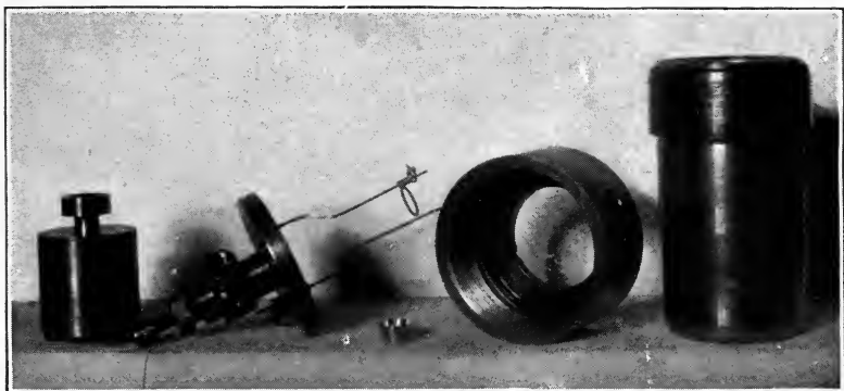
Fig. 96.—Parts of bomb calorimeter and accessories: A, pellet mold; B, cover to bomb; C, platinum dish, holding substance burned; D, collar; E, steel bomb—platinum-lined.
