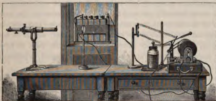
FIG. 32.—Arrangement of apparatus for observing the spectra of substances volatilised by the electric spark.
