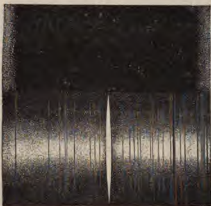
FIG. 52.—Non-coincidence of bright and dark F line when tangential slit is used, and when both photospheric and chromospheric light is admitted.
