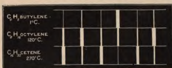
FIG. 98.—Hypothetical spectra obtained on distilling at successively increasing temperatures a mixture of light and heavy hydrocarbons.
