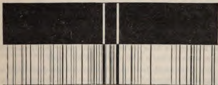
FIG. 24.—Diagram showing the solar spectrum and the bright double line D of sodium.
