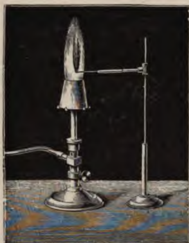
FIG. 13.—Method of inserting platinum wire and salt into flame.
