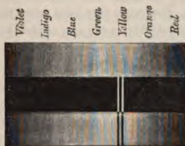
FIG. 25.—Diagram illustrating the graphical formulae employed on the opposite page. Above is the continuous spectrum given by a source of white light. Next below is the radiation spectrum (consisting of two bright lines) of sodium; and at the bottom is seen the effect of the interposition of the screen of sodium vapour between the white light and the eye. The lines are still seen occupying exactly the same positions as before, but they are reversed, i.e. they appear black on a background of continuous spectrum.
