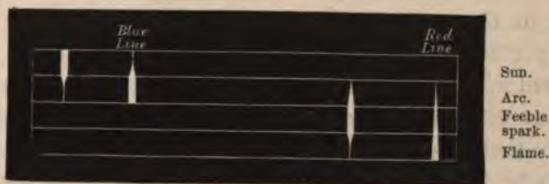
FIG. 93.—The various intensities of the lines of Lithium arranged in order of increasing temperatures.
