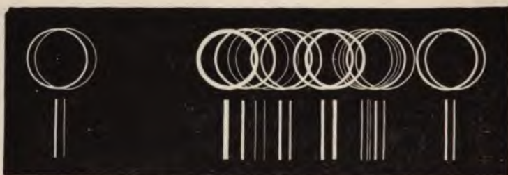
FIG. 15.—The spectrum of a complicated light-source as seen with a circular and a line slit.
