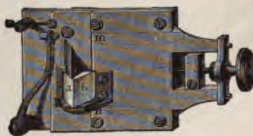
FIG. 30.—Steinheil's slit, showing reflecting prism ( a , b ).
