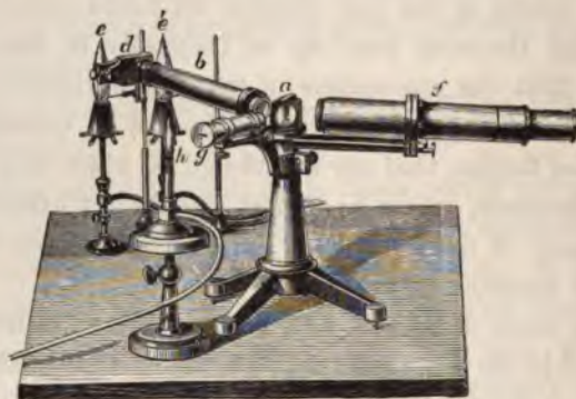
FIG. 28.—Spectroscope with reflected scale. a , prism; b , collimator; d , slit plate; e , é , Bunsen burners for volatilising salts; f , observing telescope; g , photographic scale, illuminated by gas flame, h .
