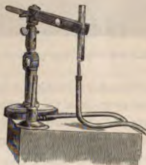
FIG. 12.—Improved Bunsen burner.
