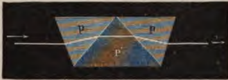
FIG. 10.—Direct-vision prism with three prisms, showing path of ray.
