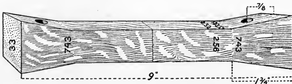
FIG. 103.—The breaking machine and test pieces used by Kahrs.
