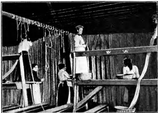
FIG. 62.—Drying room of isinglass factory. (By permission of the Bureau of Fisheries, Washington, D. C.)
