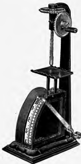
FIG. 66.—The Scott glue tester. (Kindness of The Arthur H. Thomas Company of Philadelphia.)
