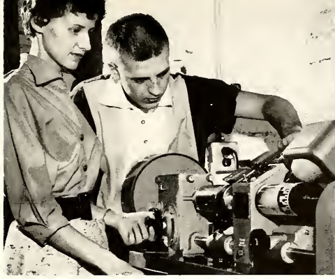
June Thomas and Joe Franko operate the Scan-a-graver which makes the Stater's plastic cuts.
