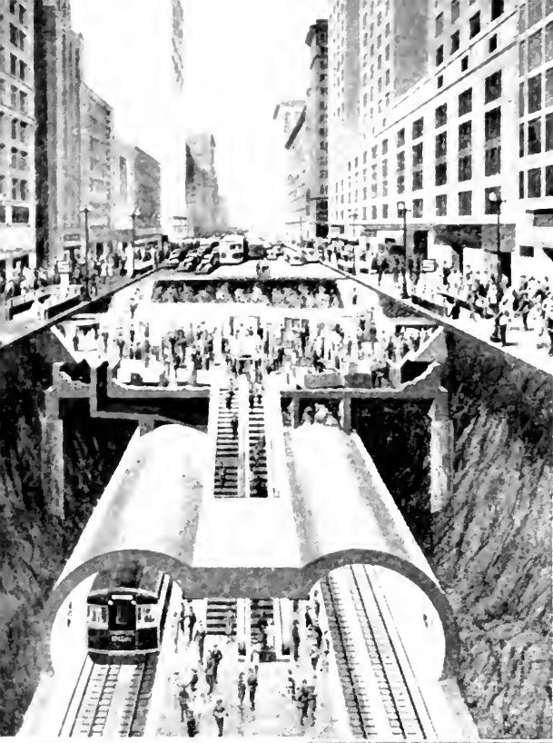
Cross section of State Street Subicay
