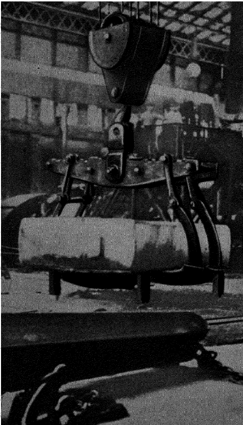
GRAPPLE. —A grapple lifting a large block of steel in a steel-rolling mill.
