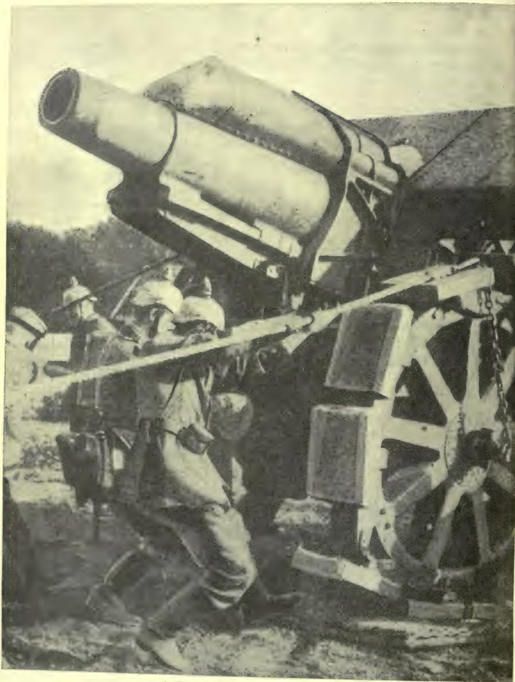
A German Howitzer for Siege Work. [ Photo, Daily Mirror. Notice the caterpillar wheels which enable it to traverse soft roads without sinking in.
