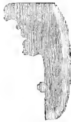
Capital of Nave Piers
