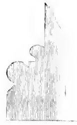
Base of Shafts, Chancel Arcade.
