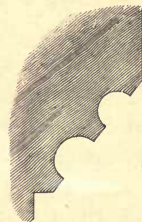
Section of Cornice round Interior.
