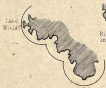
Mouldings of Arches Nave
