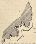
Jamb South Transept Window, interior
