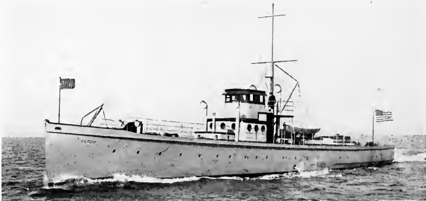
"Victory," a super-sub chaser designed by Irwin Chase, built by the Elco Works and powered with twin Standards of 500 H. P. each.
