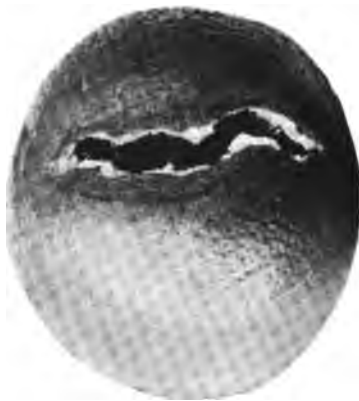
FIG. 126. — Horizontal cracks are very different from splits.
