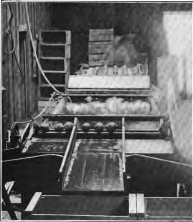
FIG. 94. — One type of water separator for frosted oranges.
